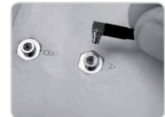
Disconnect Pigtails from the Antenna. Done :)
